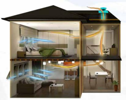
Odyssey can exchange the air in a 150m<sup>2</sup> home 6-7 times an hour all for as little as \$4.40 per month.
