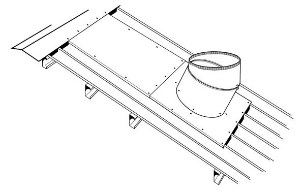
h. **Assemble Turbine:** Assemble the turbine head to the Varipitch. Re-check if the assembly is level (horizontal) and adjust the turbine by tilting the throat slightly if required. Ensure the knurling (the tapered section of the Varipitch) is fully inside the ventilator throat and secure the ventilator throat by fastening it to the top of the Varipitch with the number of fasteners shown in the table below.
