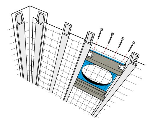
b. **Cut Hole:** Carefully cut the hole, remembering that there may be insulation and other roof members under the roof sheet. Once the hole has been cut, fold up the edge of the corrugations or pans. Ensure the roofing safety mesh/net integrity is maintained after the installation.
