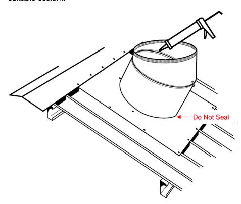
**NOTE**: **DO NOT** apply sealant to the joint between the flashing and Varipitch. This is a natural gutter to release any trapped condensation. See details in section (i) below.
