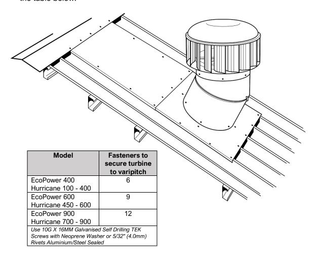
NOTE: **DO NOT** apply sealant to the joint between the turbine and Varipitch. This is a natural gutter to release any trapped condensation. See details in section (i) below.
