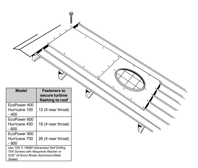
d. **Assemble the Varipitch**: When a Varipitch throat is being used, position the Varipitch on the flashing and rotate the top and bottom halves until the top of the Varipitch is level (horizontal) it is recommended that an electronic or spirit level is used to ensure that the top edge of the throat is horizontal in all directions.
