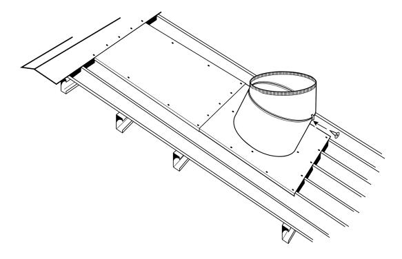
f. **Weather Sealing**: Seal the Varipitch seam on the inside with a bead of weather-resistant suitable sealant.
