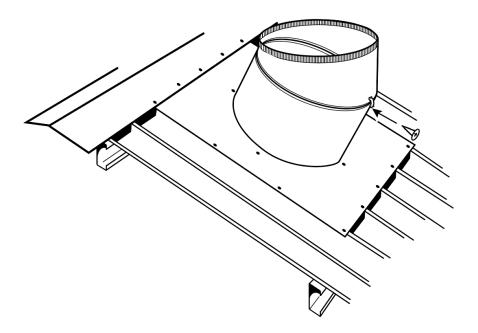
f. **Weather Sealing**: Seal the Varipitch seam on the inside with a bead of weather-resistant suitable sealant.
