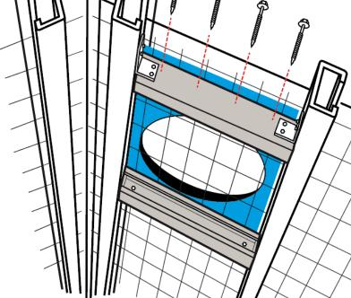
b. **Cut Hole:** Carefully cut the hole, remembering that there may be insulation and other roof members under the roof sheet. Once the hole has been cut, fold up the edge of the corrugations or pans. Ensure the roofing safety mesh/net integrity is maintained after the installation.
