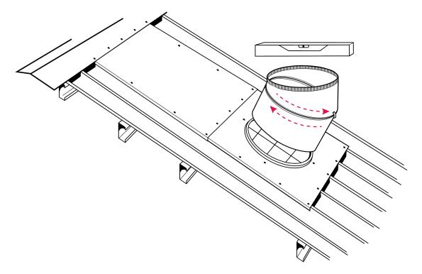
e. **Secure the Varipitch Angle:** With the Varipitch upper throat positioned horizontally, lock it into position using the supplied Varipitch clip. Use either self-tapping screws or blind rivets to secure all the clips between the two halves of the Varipitch.
