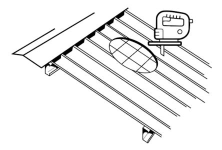
c. **Secure Flashing:** Attach the flashing under the ridge cap and using a marker draw the profile of the roof corrugation on the bottom edge of the flashing to match the roof profile.
