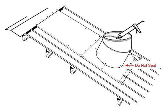
**NOTE**: **DO NOT** apply sealant to the joint between the flashing and Varipitch. This is a natural gutter to release any trapped condensation. See details in section (i) below.
