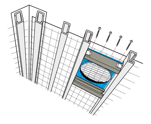
b. **Cut Hole:** Carefully cut the marked hole, remembering that there may be insulation and other roof members under the roof sheet. Once the hole has been cut, fold up the edge of the corrugations or pans to ensure there are no gaps between roof cladding and flashing. Ensure the roofing safety mesh/net integrity is maintained after the installation.
