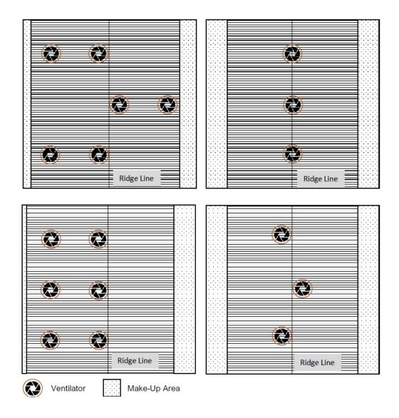
**IMPORTANT**: If external make-up air is insufficient, the ventilators will draw make-up air from each other – this will both diminish the effectiveness of the system and increase the risk of the system drawing external water into the building during periods of rain. It is also recommended that ventilators of the same size are used together to prevent replacement air from being drawn between ventilators of different sizes.
