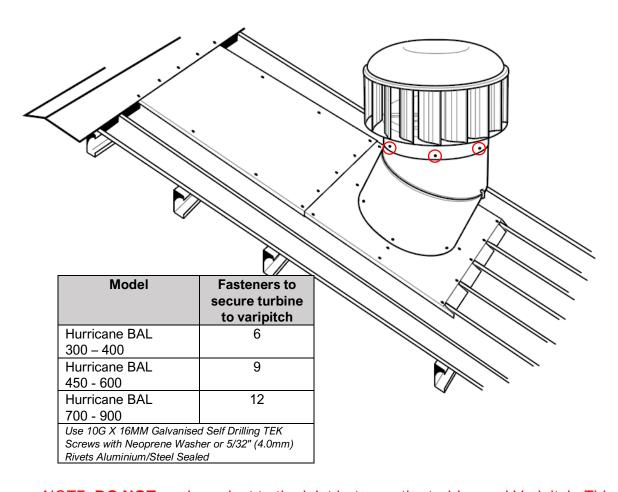
NOTE: **DO NOT** apply sealant to the joint between the turbine and Varipitch. This is a natural gutter to release any trapped condensation. See details in section (i) below.
