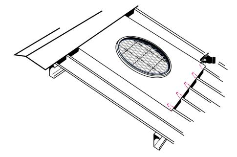
Using a pair of tin snips, cut the bottom edge of the flashing to match the roof profile. It is important to ensure that the flashing accurately matches the profile of the roof cladding with no gaps.
