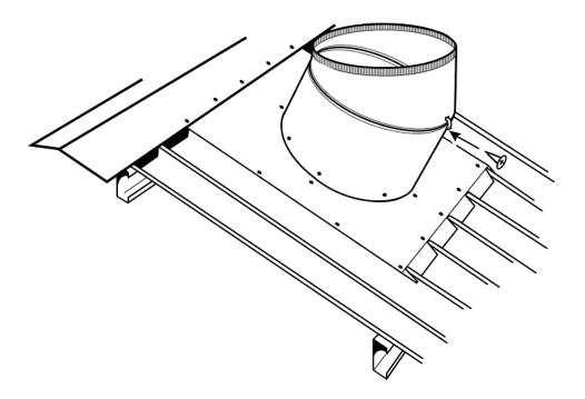
f. **Weather Sealing**: Apply sealant to all exposed screw heads and seal the Varipitch seam on the inside with a bead of weather-resistant suitable sealant.
