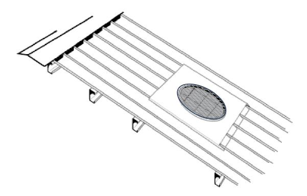
Apply sealant prior to final fixing (refer to the table below for the required number of fasteners). If trimmers are used ensure the flashing is secured to the trimmers. Seal all fasteners with a suitable sealant to ensure they are weatherproof.
