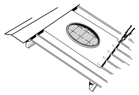
Using a soft rubber hammer, carefully work around the sides and lower edge of the flashing to form it into the corrugations of the metal sheeting profile. Care should be taken when forming the flashing so that the gaps between the roofing material and the flashing are less than 2mm.
