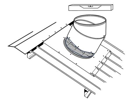
e. **Secure the Varipitch Angle:** With the Varipitch upper throat positioned horizontally, lock it into position using the supplied Varipitch clip. Use either self-tapping screws or blind rivets to secure all the clips between the two halves of the Varipitch.
