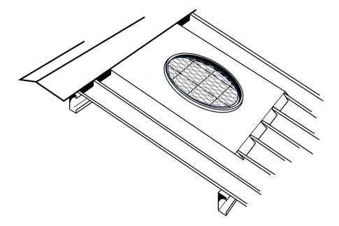
Apply sealant prior to final fixing (refer to the table below for the required number of fasteners). If trimmers are used ensure the flashing is secured to the trimmers. Seal all fasteners with a suitable sealant to ensure they are weatherproof.
