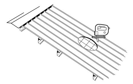
c. **Secure Flashing:** Attach the flashing over the roof hole and using a marker draw the profile of the roof corrugation on the bottom edge of the flashing to match the roof profile.
