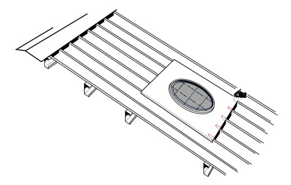
Using a pair of tin snips, cut the bottom edge of the flashing to match the roof profile. This will help ensure the lower profile of the roof covered by the flashing.
