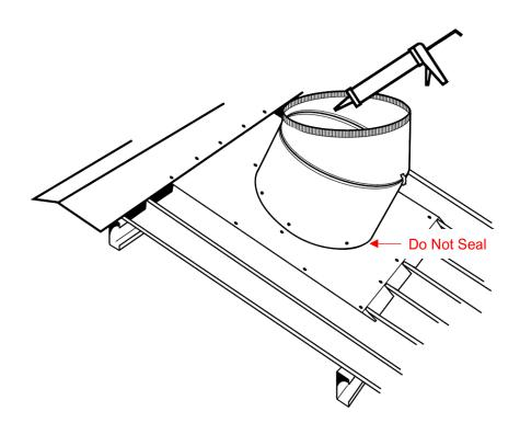
**NOTE**: **DO NOT** apply sealant to the joint between the flashing and Varipitch. This is a natural gutter to release any trapped condensation. See details in section (i) below.
