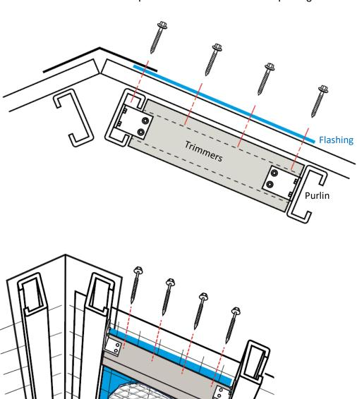
b. **Cut Hole:** Carefully cut the marked hole, remembering that there may be insulation and other roof members under the roof sheet. Once the hole has been cut, fold up the edge of the corrugations or pans to ensure there are no gaps between roof cladding and flashing. Ensure the roofing safety mesh/net integrity is maintained after the installation.
